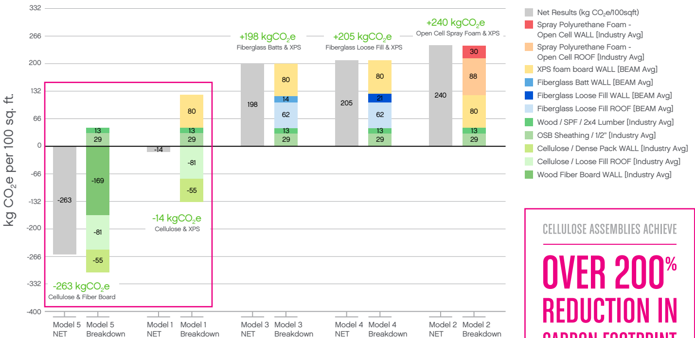
Carbon Footprint Comparison of 5 Identical Assemblies 3 R-13 Cavity Insulation, R-10 Continuous Insulation, R-38 Attic Insulation
