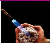
With a flame spread of 25 or less, Greenfiber has a Class 1 Fire rating. Walls with Greenfiber insulation are one-hour (or greater) fire walls and can help control the spread of fire. Greenfiber also has a very low smoke development index level.
