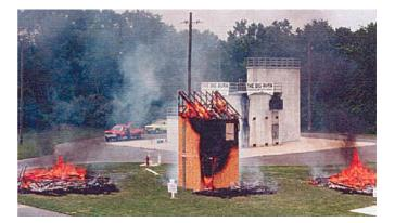
The results of this demonstration correspond closely with the results achieved by the National Fire Laboratory of the National Research Council Canada. The cellulose insulation structure maintained its structural integrity, for a total time of 68.08 minutes, in excess of 24 minutes longer than the fiberglass structure or the uninsulated structure translating to an increased fire resistance of 57% as compared to the 55% improvement achieved in the laboratory study.
