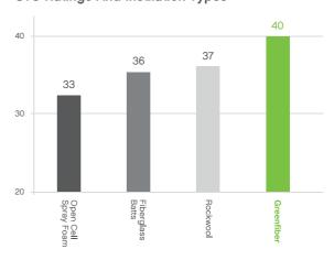
Note: Based on STC ratings for the same assembly for Owens Corning 3.5" Quiet Zone Batt, Rockwool 3.5" Comfortbatt, Huntsman 2" Class Plus Open-cell spray foam, Greenfiber 3.5" dense-pack cellulose.
