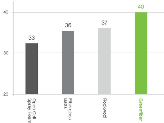
Note: Based on STC ratings for the same assembly for Owens Corning 3.5" Quiet Zone Batt, Rockwool 3.5" Comfortbatt, Huntsman 2" Class Plus Open-cell spray foam, Greenfiber 3.5" dense-pack cellulose.
