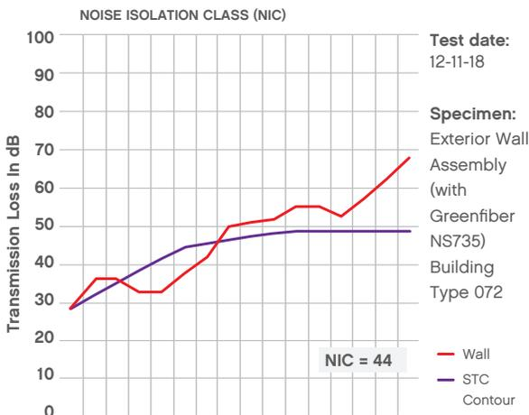
\* Field STC testing was completed using NIC methodology.
