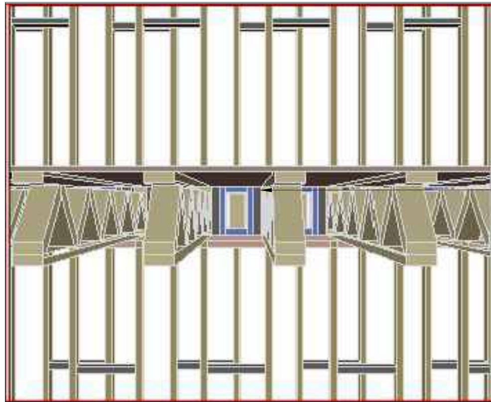
NON-STEPPED CONDITION - OPEN WEB FLOOR JOISTS
