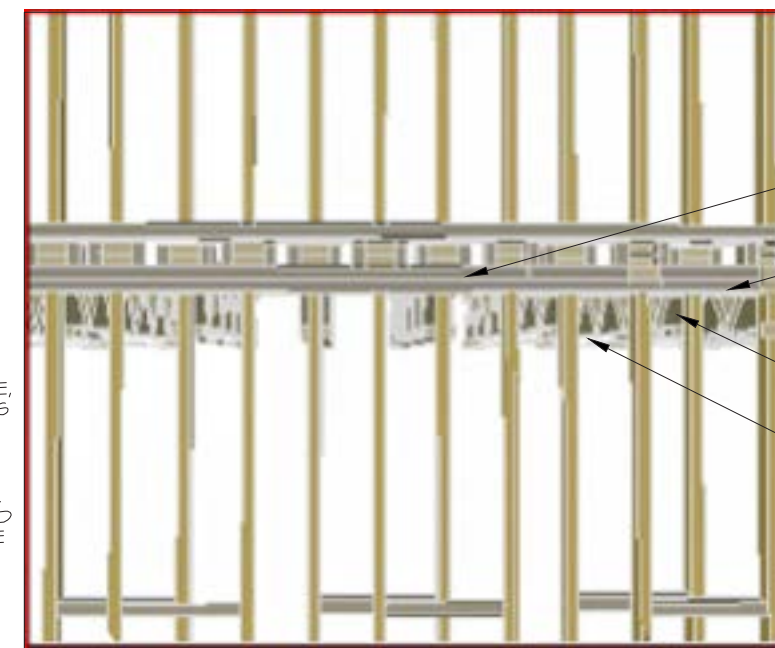
STEPPED CONDITION - TOP CHORD LOAD BEARING FLOOR JOISTS
