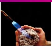
With a flame spread of 25 or less, Greenfiber has a Class 1 Fire rating. Walls with Greenfiber insulation are one-hour (or greater) fire walls and can help control the spread of fire. Greenfiber also has a very low smoke development index level.
